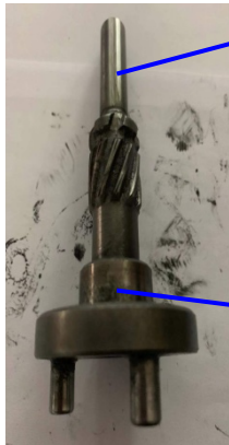
滚珠、扭簧未见变形 No deformation of spring and drive roller
