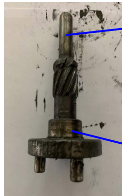
滚珠、扭簧未见变形 No deformation of spring and drive roller
