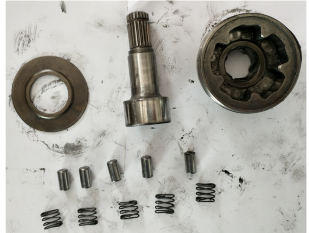
滚珠、扭簧未见变形 No deformation of spring and drive roller
